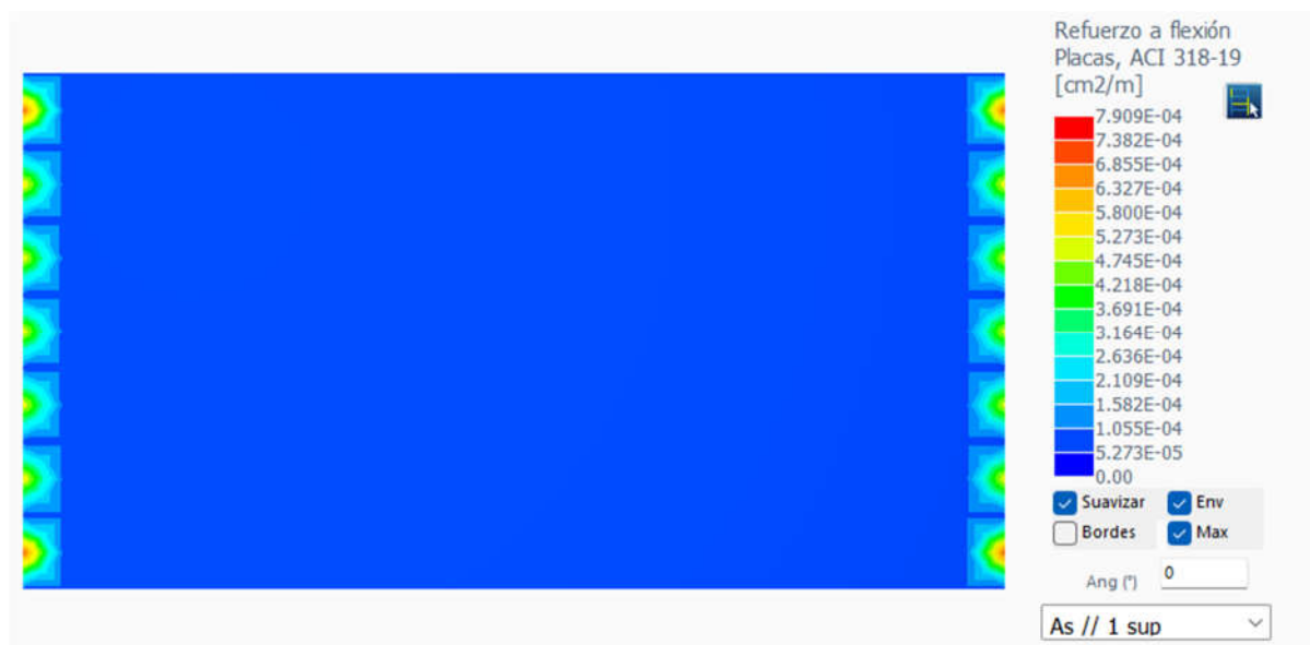
Figura N° 7 – Armadura As // 1 Sup.
